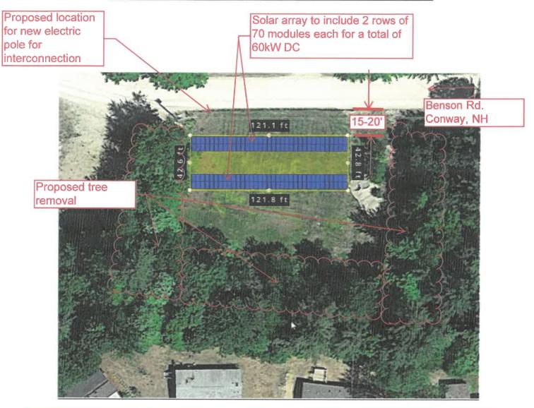
NOTES: No fence is proposed because the back of the array and all wiring will be covered with a wire mesh so that there is no access to any wiring.
